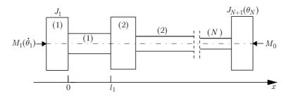
Fig. 1. Discrete-continuous multi-mass torsional system
