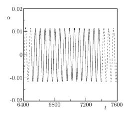
Fig. 6. Comparison of numerical (dashed line) and analytical solutions (continuous line) for displacements of the three-mass system in x = 2 in a steady state with boundary condition (3.3) and  $\Omega_0 = 0.05$
